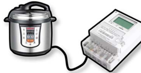
EPCs connected to A2EI Smart Meters
