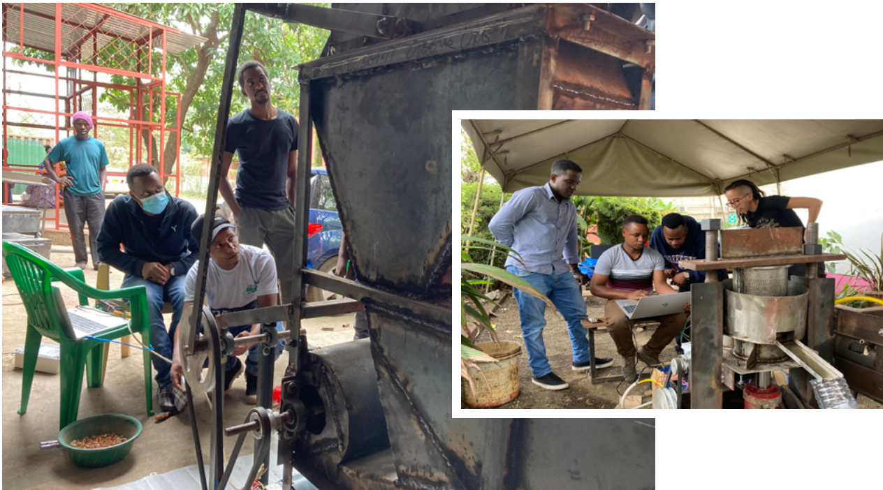
A2EI and Imara Tech teams testing a solar-powered peanut sheller (left) and solar-powered oil press (right).
