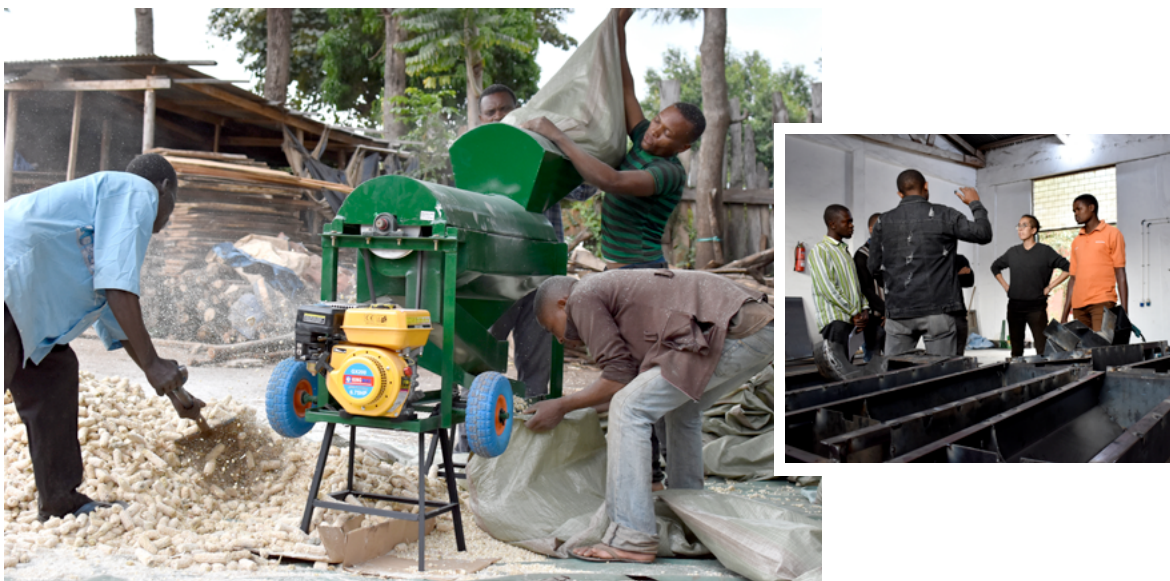
Customers operate the MCT for threshing crops such as maize (left). The threshers are made locally at the Imara Tech workshop (right).
