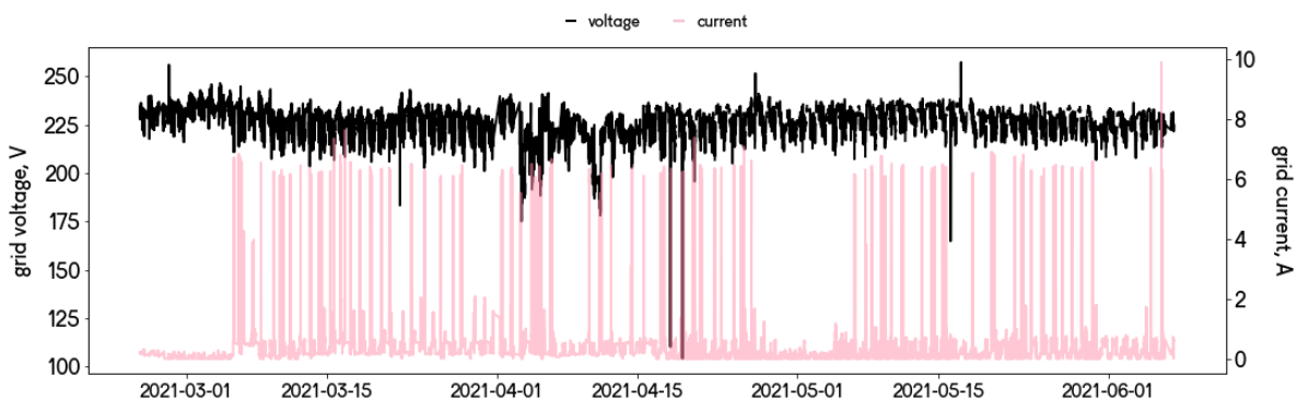
Fig. 9: This is the voltage and current values from the grid meter with no. 86000005 in household no. 4.
